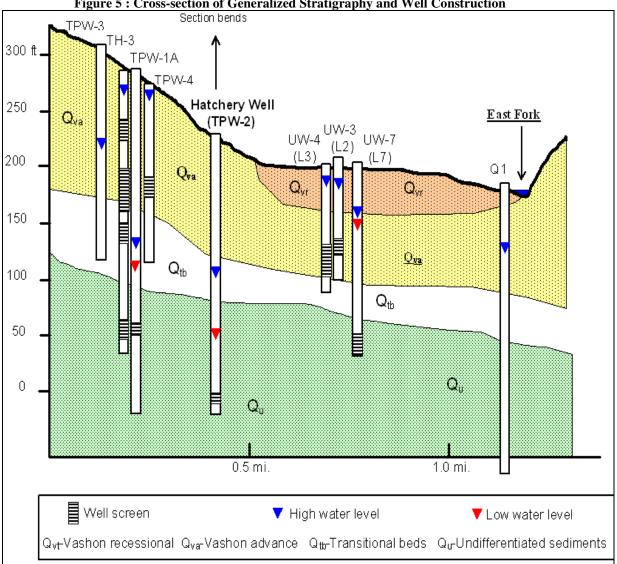
Figure 5 : Cross-section of Generalized Stratigraphy and Well Construction
